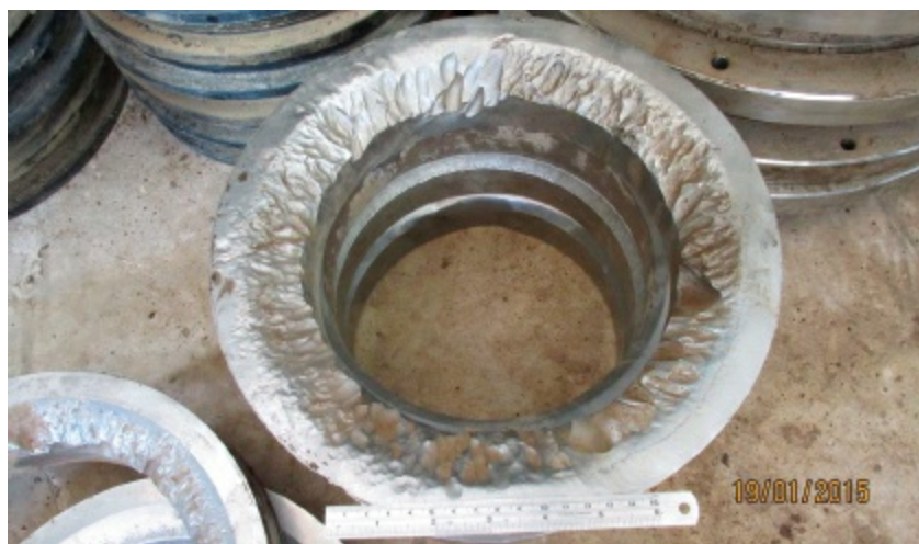
FIGURE 1.3: A 2205 valve seat after 4 days operation.
