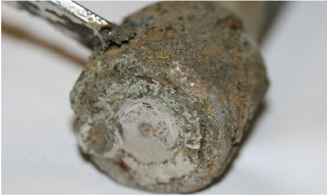
FIGURE 1.1: A 2205 duplex stainless steel agitator after a few days exposure to a hot, chloride-rich, acidic bioleach slurry.
