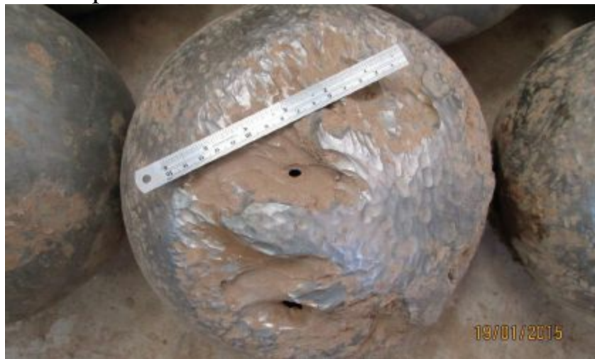
FIGURE 1.2: A 316Ti ball from a positive displacement pump after 4 days operation. The original wall thickness was 20mm.
